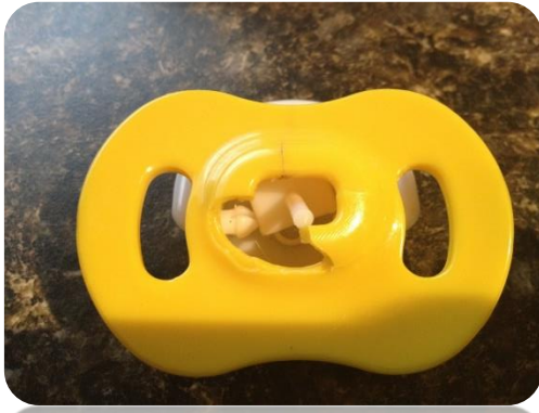
Figure 3: A pacifier with a broken plastic base. Small broken pieces can be ingested and children can choke on them (from SaferProducts.gov).
