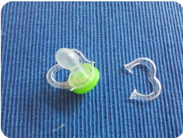
Figure 2: A broken plastic pacifier. These sharp plastic edges pose a laceration risk when they break inside or around a child's mouth (from themommahen.wordpress.com ).
